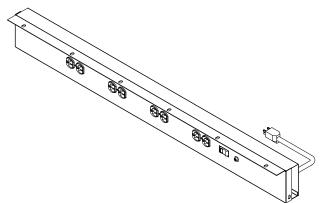
**2.** Attach the wireway cover to the outlet panel with four #10 sheet metal screws.
