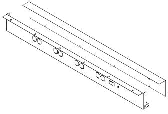
**3.** Place the outlet panel under the bench top and between the modular units. Position the outlet panel flange flush with the front edge of the top, aligning the holes in the flange with the holes in the top. Secure with six 1/4"-20 x 5/8" bolts.
