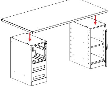
**4.** Position the top so that the ends of the top are flush with the side of the cabinets, then tighten all the bolts. Replace the drawers and/or close the cabinet doors.
