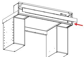
**4.** Attach the back rail to the side rails, using two 1/4"-20 x 5/8" bolts and nuts on each end.
